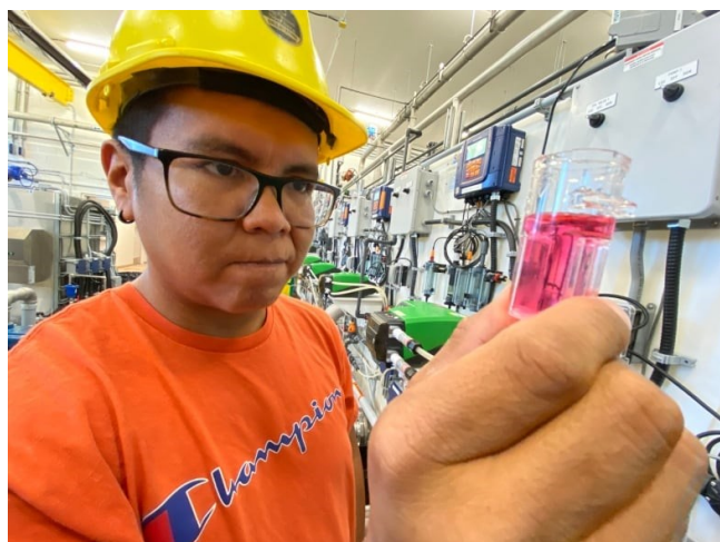
Green, the Shoal Lake 40 water treatment plant operator, tests for chlorine. (Tyson Koschik/CBC)
