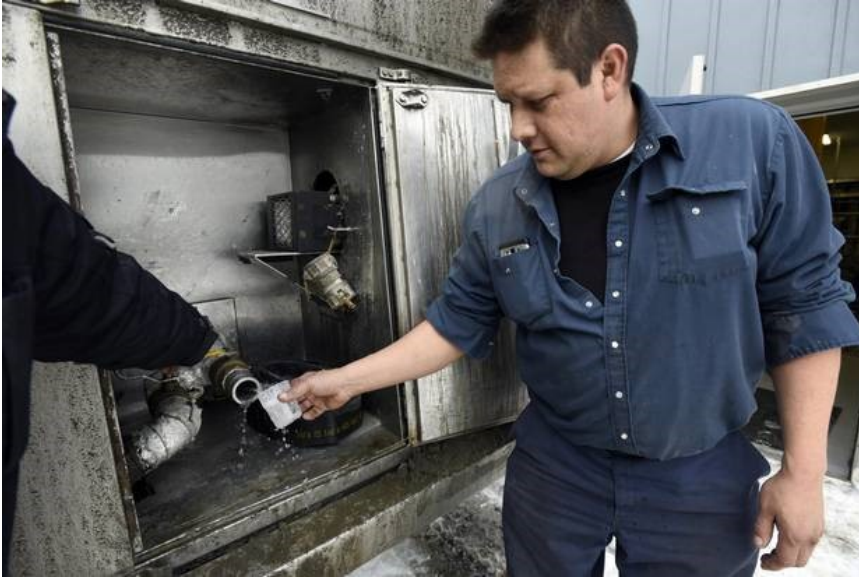
John Owl, an infrastructure technician, takes a sample from a tanker delivering fresh water before it can be transferred to reservoirs on the Serpent River First Nation on December 19, 2016.
